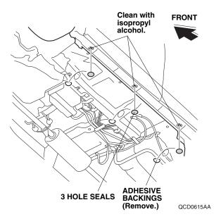
29. Remove the adhesive backing from each hole seal, and attach the seal over the holes as shown.
