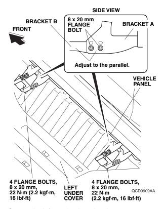
Secure the left running board to the two brackets A. Torque the flange bolts: 22 N⋅m (2.2 kgf⋅m, 16 lbf⋅ft).
