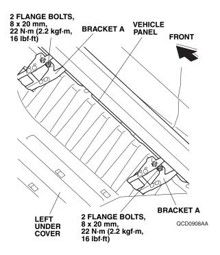
48. Secure the two brackets A to the two brackets B. Torque the flange bolts: 22 N·m (2.2 kgf·m, 16 lbf·ft).
