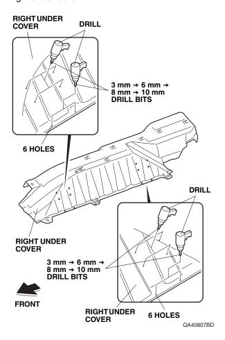
27. While wearing eye protection and using an air saw, cut the right under cover as shown. Remove any burrs.
