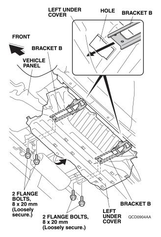
43. With help from an assistant place the left under cover close to the vehicle and loosely install the two brackets B to the vehicle panel using four 8 x 20 mm flange bolts.
