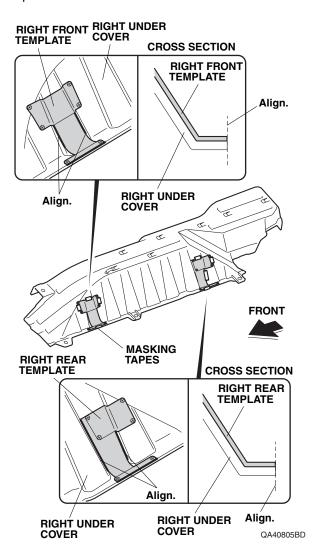
24. Using a pushpin, pierce six marks on the each templates.
