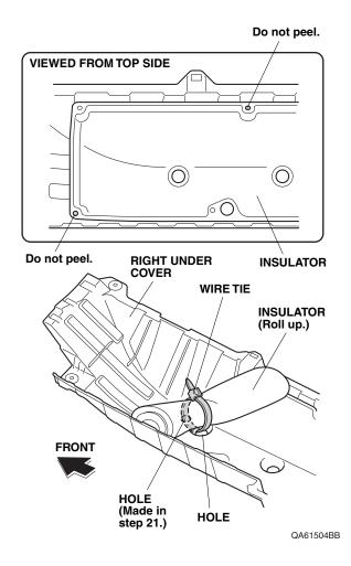
23. Align and attach the right front template and right rear template to the right under cover with masking tapes.
